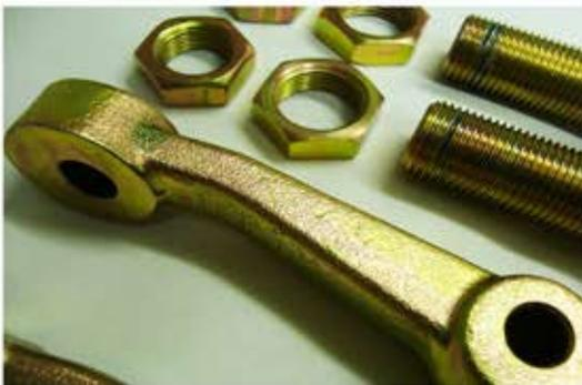
AFT offers over 16 quality specified plating processes, including: silver, black oxide, zinc nickel, phosphate, tin, matte tin, and Xylan® Coatings.
